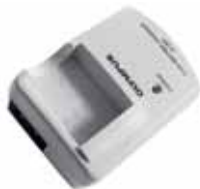
LI-30C Quick charger Charger for the LI-30B lithium-ion battery.
