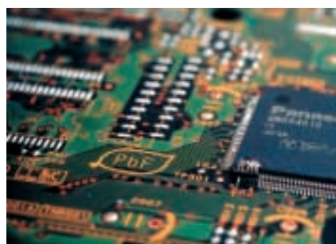
LEAD-FREE PRINTED CIRCUIT BOARD WITH LEAD-FREE SOLDER
