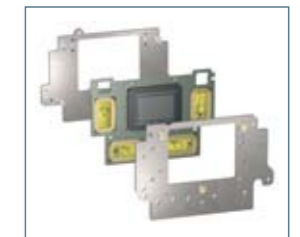
CCD plate with electromagnets to control the "Shake Reduction" mechanism is connected to permanent magnets to the metal frame as a unit.
