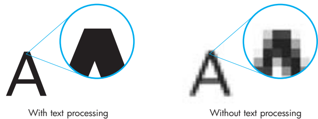
Text processing eliminates vertical and horizontal scaling distortion and minimises ringing
